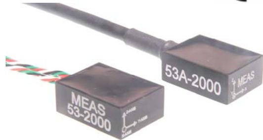
**The Model 53 Accelerometer** is a small, compact triaxial device designed for vehicle impact and road testing. The accelerometer incorporates gas-damped MEMS sensing elements with mechanical stops for high overload protection. Featuring ranges from  $\pm 50g$  to  $\pm 2000g$  and frequency response to 5000Hz, this sensor is easily mounted in hard to reach places on vehicles under test.
